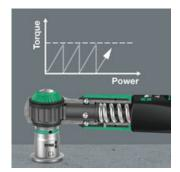
The Safe-Torque A 1 torque wrench is equipped with a slide-over mechanism. Once the set torque value has been reached, the tool cannot be overtightened, so that excessive torque cannot be applied.
